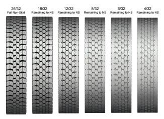
\*Diagram depicts a simulation of tread pattern evolution, not an actual representation of wear rates. Actual results may vary based upon a number of factors including, but not limited to, types of vehicles, road conditions, driving habits, tire inflation, vehicle loads and temperature. Proper application and regularly scheduled maintenance must occur for best results.
